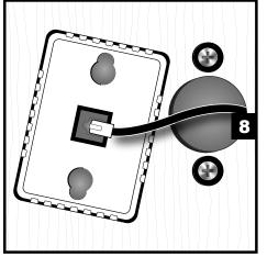
Plug the data cable into the back of the wall control.
