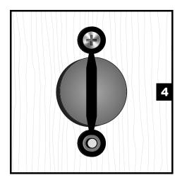
Install one (1) screw in the TOP mounting tab. Do not completely tighten.
