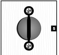
Make sure tabs are perpendicular to the floor and install the remaining screw in the BOTTOM mounting tab. Tigthen both screws.
