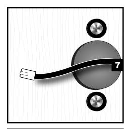
Route the data cable through the 1 1/4" cut hole in STEP 1.
